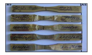
Fig. 10. The macro images of fatigue fracture zones.
