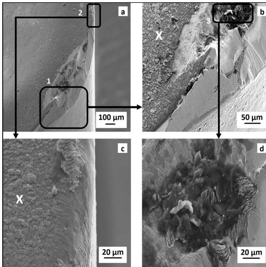
Fig. 6. The SEM images of cutting insert after milling of specimen M1 with parameters of  $V_c = 120 \text{ m min}^{-1}$ ,  $f_z = 0.02 \text{ mm/tooth}$ .
