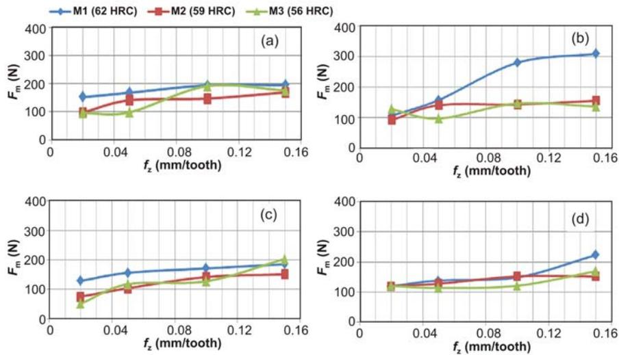
Fig. 5. Changing of  $F_m$  according to the feed rate at four different cutting speeds:  $60 \text{ m min}^{-1}$  (a),  $80 \text{ m min}^{-1}$  (b),  $100 \text{ m min}^{-1}$  (c),  $120 \text{ m min}^{-1}$  (d).
