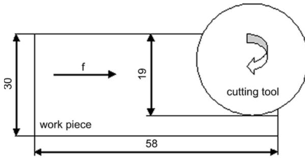
Fig. 1. Work piece and milling method.
