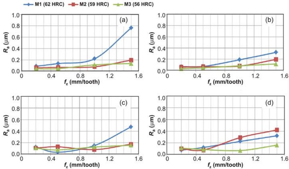
Fig. 4. Changing of  $R_a$  according to the feed rate at four different cutting speeds:  $60 \text{ m min}^{-1}$  (a),  $80 \text{ m min}^{-1}$  (b),  $100 \text{ m min}^{-1}$  (c),  $120 \text{ m min}^{-1}$  (d).
