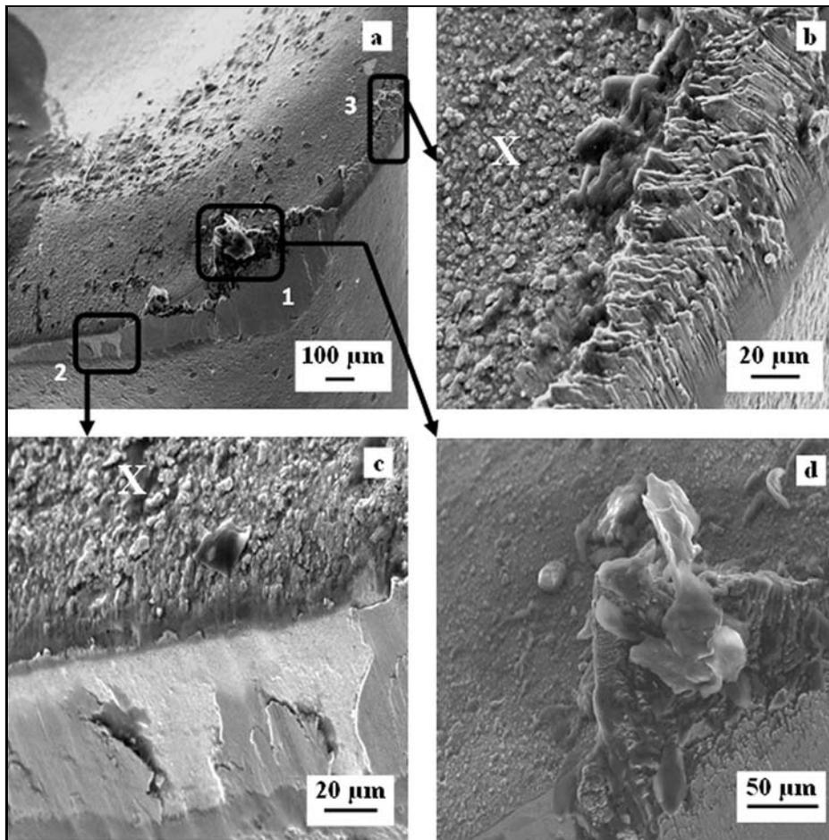
Fig. 7. The SEM images of cutting insert after milling of specimen M2 with parameters of  $V_c = 120 \text{ m min}^{-1}$ ,  $f_z = 0.02 \text{ mm/tooth}$ .
