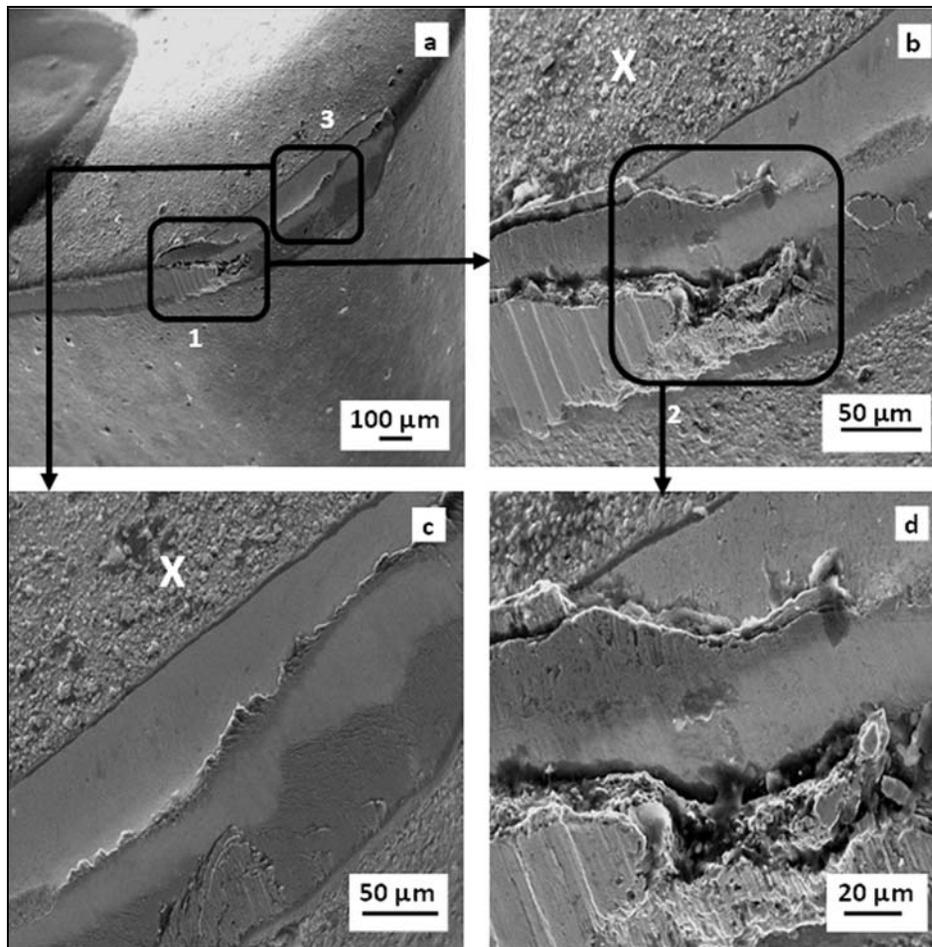
Fig. 8. The SEM images of cutting insert after milling of specimen M3 with parameters of  $V_c = 120 \text{ m min}^{-1}$ ,  $f_z = 0.02 \text{ mm/tooth}$ .
