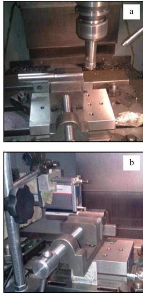
Fig. 3. Performing of experiment in machine (a), measuring of surface roughness (b).
