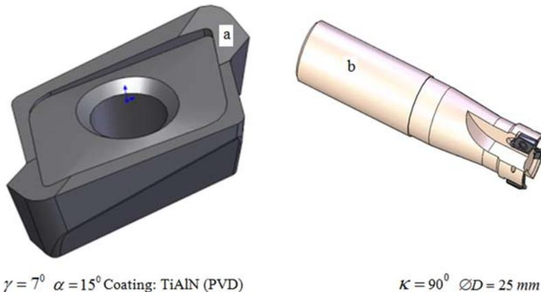
Fig. 2. Form and dimensions of the cutting insert used in the experiments (a), tool holder (b).
