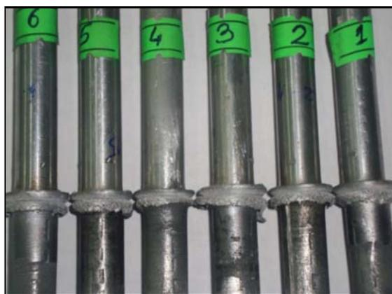
Fig. 2. Overview of friction welded SiCp reinforced aluminum composite to AA 6061 alloy.
