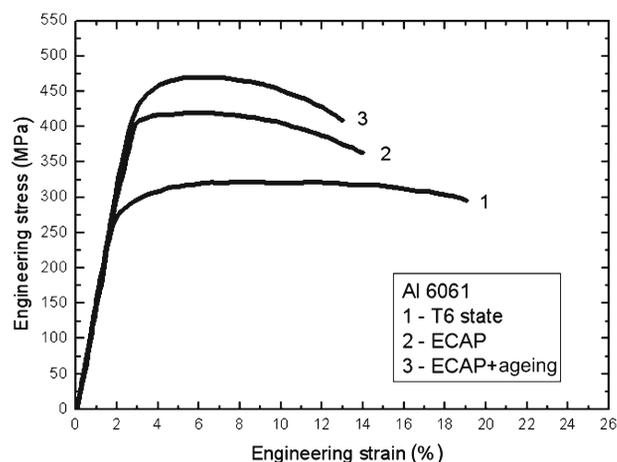
Fig. 1. Stress-strain plot of the 6061 aluminium alloy T6 treated, processed by ECAP in the solution treated state and processed by ECAP followed by additional ageing.
