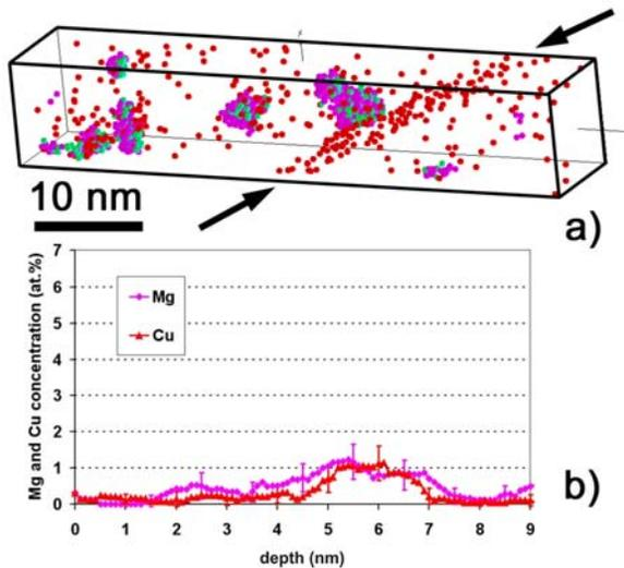
Fig. 3. (a) 3D reconstruction ( $10 \times 10 \times 55 \text{ nm}^3$ ) of a volume analysed in the 6061 aluminium alloy processed by ECAP. The data set was filtered to exhibit Mg rich nanoscaled precipitates (Mg pink, Si green and Cu red). Additionally, all Cu atoms detected in the volume are plotted to show segregation along a planar boundary (arrowed); (b) composition profile computed across this boundary showing a significant segregation of Cu and Mg (sampling volume thickness 1 nm).
