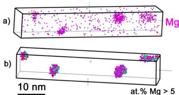
Fig. 4. 3D reconstruction ( $10 \times 10 \times 60 \text{ nm}^3$ ) of a volume analysed in the 6061 aluminium alloy processed by ECAP followed by ageing during 24 h at  $130^\circ\text{C}$ . (a) Distribution of all detected Mg atoms showing nanoscaled spherical precipitates; (b) filtered data with another orientation (Mg atoms pink, Si atoms green and Cu atoms red).
