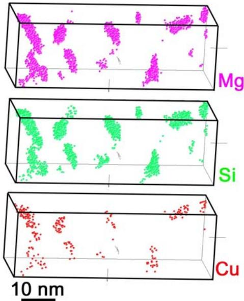
Fig. 2. 3D reconstruction ( $20 \times 20 \times 60 \text{ nm}^3$ ) of a volume analysed in the T6 treated 6061 aluminium alloy. The data set was filtered to exhibit Mg rich nanoscaled precipitates. The distribution of Mg, Si and Cu is displayed on three different images.
