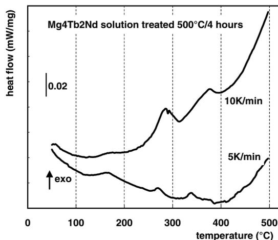
Fig. 2. DSC curves of Mg<sub>4</sub>Tb<sub>2</sub>Nd alloy solution treated at 500°C/4 hours at heating rates 5 K min<sup>-1</sup> and 10 K min<sup>-1</sup>.
