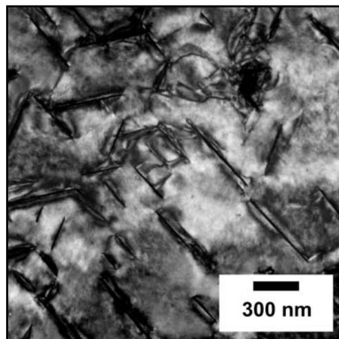
Fig. 4. Triangular arrangement of  $\beta_1$  prismatic plates parallel to  $\{10\bar{1}0\}_{\text{Mg}}$  planes in Mg<sub>4</sub>Tb<sub>2</sub>Nd alloy annealed up to 330°C.
