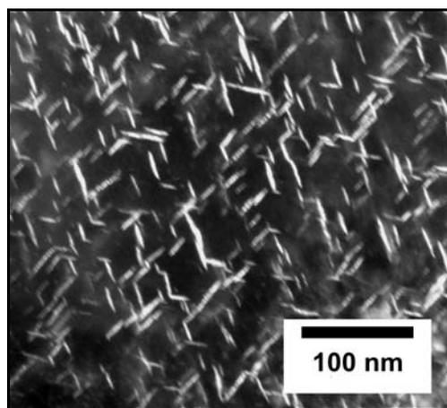
Fig. 3. Triangular arrangement of D<sub>019</sub> phase prismatic plates parallel to  $\{11\bar{2}0\}_{\text{Mg}}$  planes in Mg<sub>4</sub>Tb<sub>2</sub>Nd alloy annealed up to 270°C.
