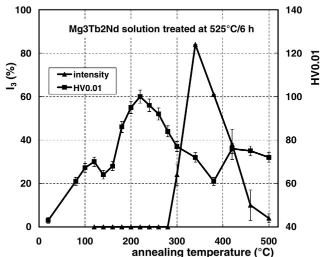
Fig. 5. Intensity development of positrons trapped at precipitate interfaces and microhardness development with isochronal annealing (20 K/20 min) of Mg<sub>3</sub>Tb<sub>2</sub>Nd alloy solution treated at 525 °C/6 hours.
