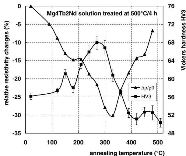
Fig. 1. Resistivity at 77 K and hardness response on isochronal annealing of Mg<sub>4</sub>Tb<sub>2</sub>Nd alloy solution treated at 500 °C/4 hours.
