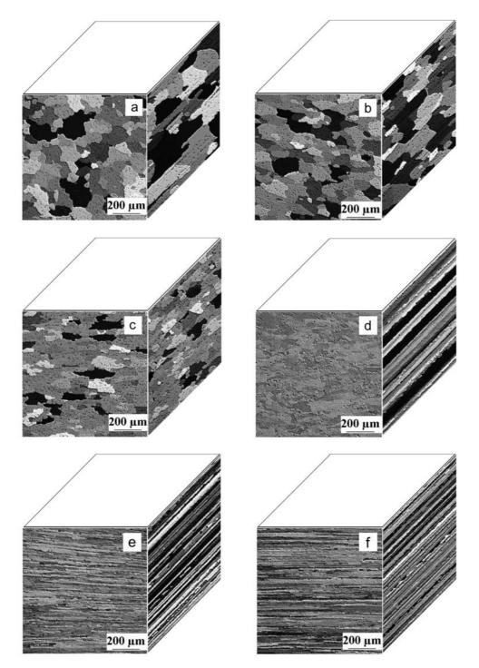
Fig. 2. Micrographs of aluminium alloys: AlMg3 from a) position 1, b) position 2, c) position 3 and AlCuMgLi from d) position 1, e) position 2, f) position 3.
