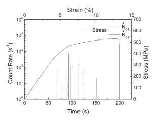
Fig. 6. Stress-strain and AE count rate-time curves of 1441 alloy, position 3.
