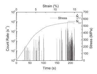
Fig. 7. Stress-strain and AE count rate-time curves of 1441 alloy, position 4.
