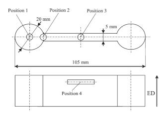
Fig. 1. Schematical drawing of extruded profile with setting out of sample positions.
