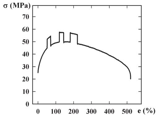
Fig. 10. Dependence of true stress on strain for the material strained at 623 K and the initial strain rate of  $2 \times 10^{-2} \text{ s}^{-1}$ .
