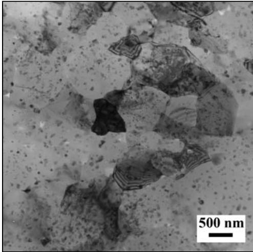
Fig. 6. Microstructure of material annealed for 1 h at 723 K, regions with 500 nm grains can still be found.
