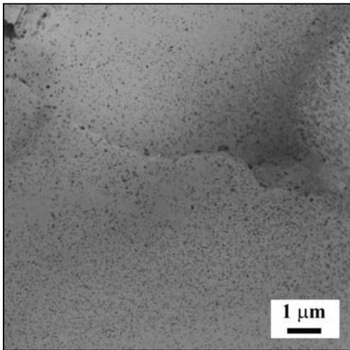
Fig. 7. Microstructure of material annealed for 1 h at 723 K, grains coarsened to 10 μm, occasionally even more, as documented in Fig. 7.
