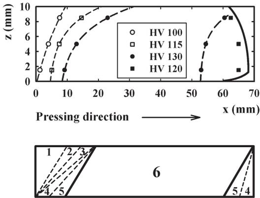
Fig. 2. Microhardness on the side plane of the ECAP billet compared with the theoretical position of the DDZ.
