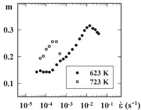
Fig. 9. Dependence of the strain rate sensitivity parameter on true strain rate.
