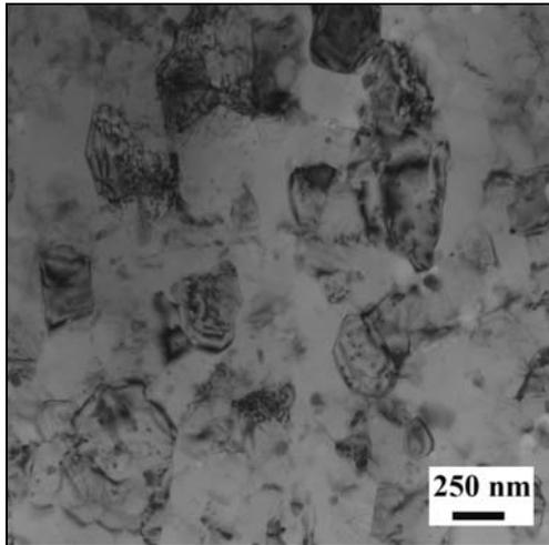
Fig. 3. Microstructure of material in the initial state after ECAP.
