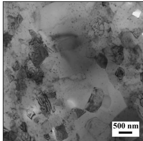
Fig. 5. Microstructure of material annealed for 1 h at 623 K, local bands of coarser grains are starting to appear.
