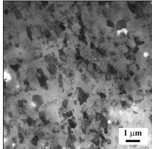
Fig. 4. Microstructure of material annealed for 1 h at 623 K, sub-micrometer grains in a large part of the volume.
