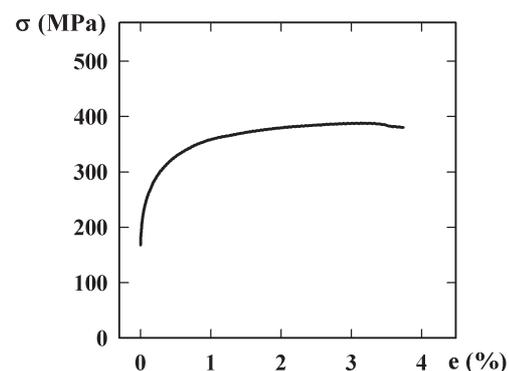
Fig. 1. True stress vs. strain dependence at room temperature and an initial strain rate of  $1 \times 10^{-4} \text{ s}^{-1}$ .
