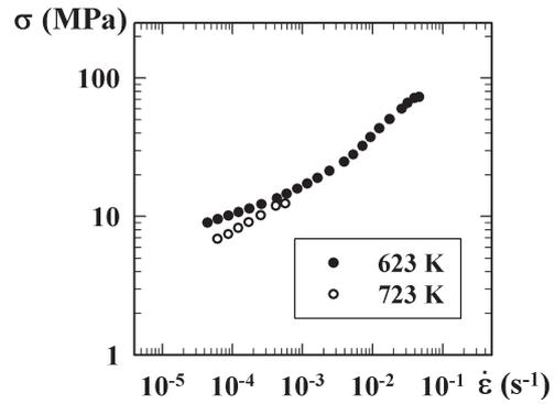
Fig. 8. Dependence of true stress on true strain rate.
