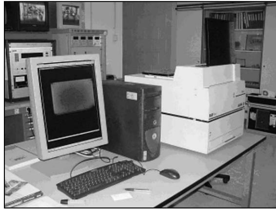
Fig. 2. The system for digital radiography consists of a scanner AGFA RadView CR100 for digitization of the imaging plates, computer with dedicated software and high-resolution monitor.
