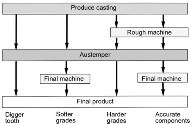
Fig. 9. Options for integrating casting, machining and heat treatment of ADI components.
