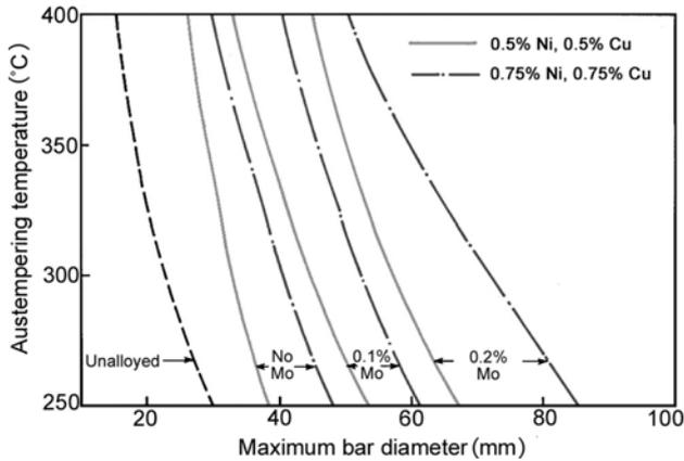
Fig. 4. Effect of combinations of Ni, Cu and Mo on the maximum bar diameter that can be austempered without the formation of pearlite [9].
