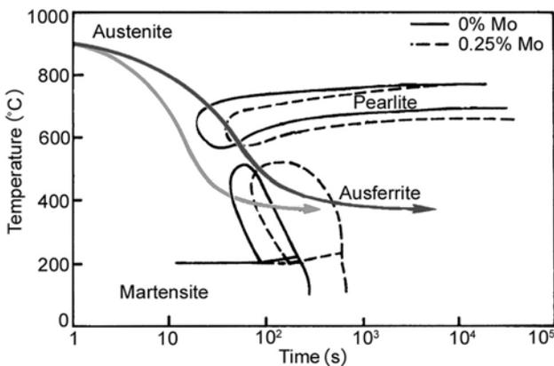
Fig. 2. CCT diagrams for 3.3% C, 2.6% Si, 0.3% Mn ductile iron with superimposed cooling curves.
