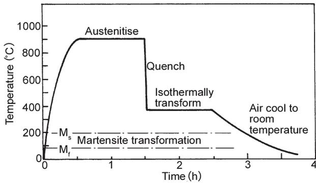
Fig. 1. Typical austempering cycle used for ductile irons.
