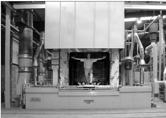
Fig. 8. Austempering furnace recently installed in the UK [17]. Courtesy of ADI Treatments Ltd., UK.
