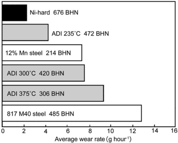
Fig. 18. Impact erosion wear tests on ADI and competing materials [8].
