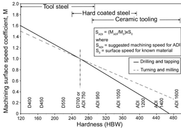
Fig. 10. Suggested tool materials and machining conditions for ADI [33]. Courtesy of Applied Process Inc.
