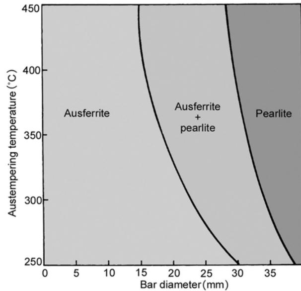
Fig. 3. The effects of austempering temperature and bar diameter on the microstructures produced at the bar centre.
