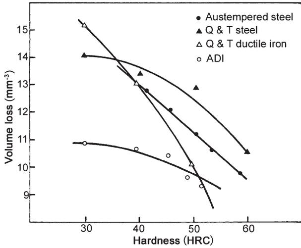
Fig. 17. Pin abrasion wear tests on ADI, ductile iron and two steels [8].
