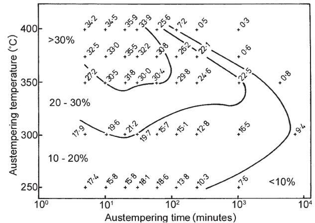
Fig. 14. Effect of austempering parameters on the retained austenite content. Ductile iron alloyed with 1% Ni [45].
