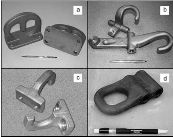
Fig. 25. ADI towing hooks for (a) Jeep Liberty, (b) GM, (c) Chevy Equinox, (d) Hummer. Courtesy of Applied Process Inc.
