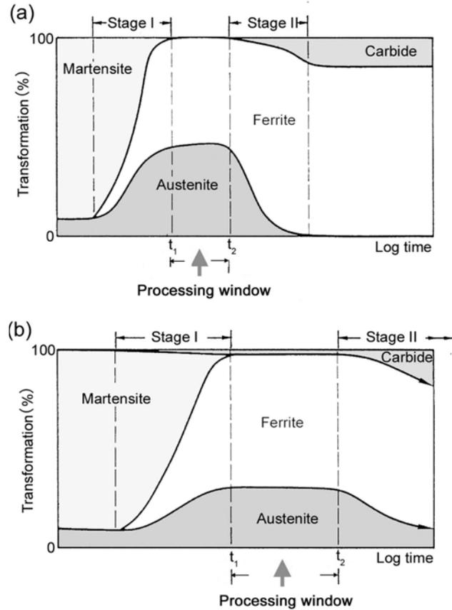
Fig. 6. Developments in the microstructure when austempering ductile iron at (a) high temperatures, (b) low temperatures. After Voigt [15].
