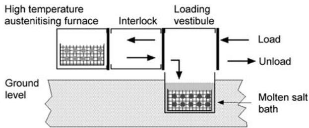
Fig. 7. Schematic view of an 'atmosphere-to-salt' austempering furnace.
