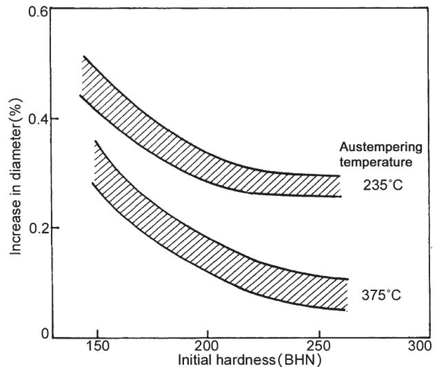
Fig. 5. Effect of initial structure and austempering temperature on the change in diameter of a 150 mm diameter disc [9].
