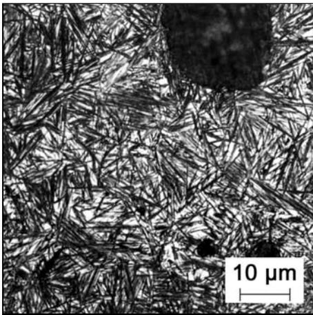
Fig. 12. Typical microstructure obtained by austempering at a low temperature (260 °C).
