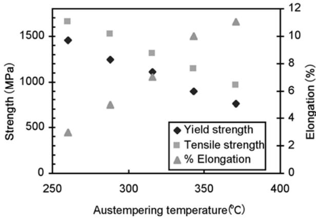
Fig. 11. Typical tensile properties of ADI as a function of the austempering temperature. Based on data from Rundman [44].
