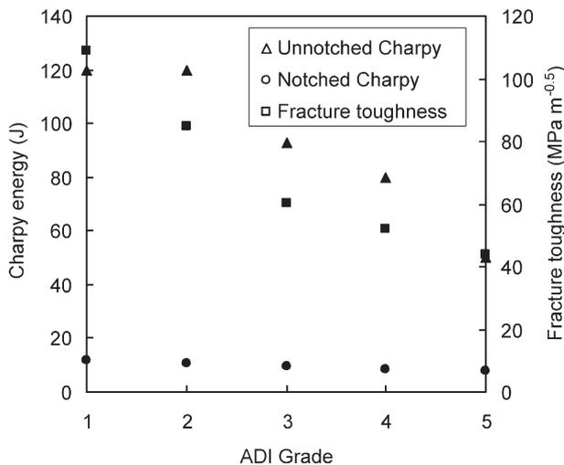
Fig. 16. Typical values of the impact and fracture toughness properties of ASTM A897M-03 grades of ADI using data from [50].
