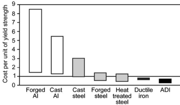
Fig. 20. Comparison of the cost per unit of yield strength for different materials. Courtesy of Applied Process Inc.
