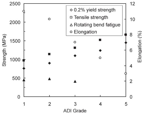
Fig. 15. Typical values of the tensile and fatigue properties of ASTM A897M-03 grades of ADI using data from [50].
