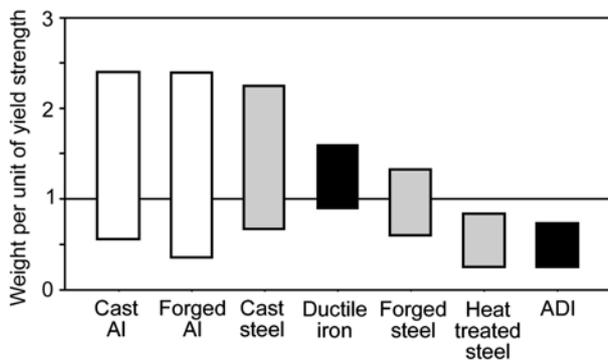
Fig. 21. Comparison of the weight per unit of yield strength for different materials. Courtesy of Applied Process Inc.
