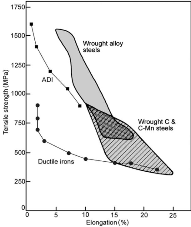
Fig. 19. Comparison of the minimum tensile properties of ADI (ASTM A897M-03), ductile irons (EN1563:1977) and forged steels (BS970:1983).
