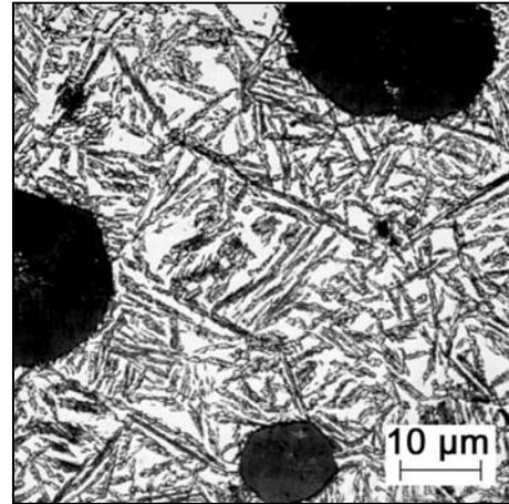
Fig. 13. Typical microstructure obtained by austempering at a high temperature (375 °C).
