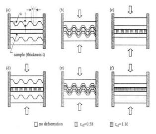
Fig. 2. A schematic illustration of CGP method [1].
