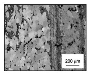
Fig. 1. LOM micrograph of initial recrystallized structure of aluminium.
