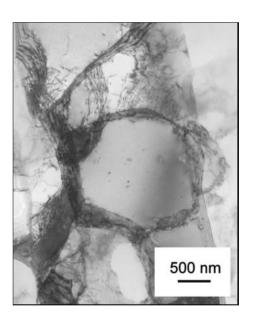
Fig. 12. Formation of new grains by dislocation rearrangement (3-A-TEM).
