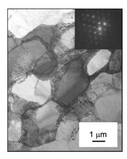
Fig. 9. TEM micrograph formation of new grains with high angle boundaries (2-B-TEM specimen).
