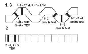
Fig. 4. Shapes of the 3 plate specimens and locations of TEM and tensile test samples.
