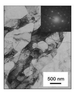
Fig. 8. TEM micrograph of polygonized structure (1-B-TEM specimen).
