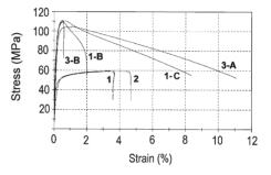
Fig. 13. Mechanical properties of specimens. No. 1 and 2 denote the initial as-annealed plate, whilst the remaining curves correspond to tensile specimens as shown in Fig. 4.
