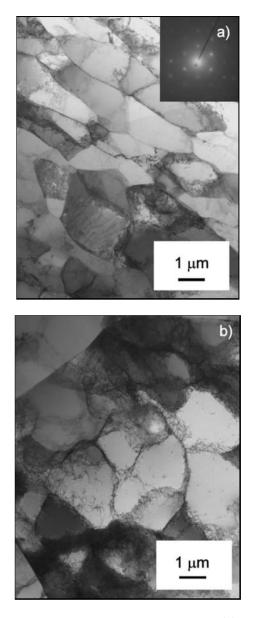
Fig. 5. TEM micrograph of subgrain structure (a) and dislocation cell structure (b) formed in the flat area of the grooved plate (segment 1-A-TEM).
