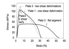
Fig. 14. Records of tensile tests performed with small specimens for different segments of plates.
