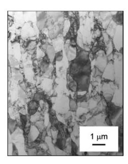
Fig. 10. TEM micrograph of subgrains microstructure after second pressing between grooved dies (3-A-TEM).
