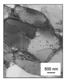
Fig. 6. TEM micrograph of high-angle grain boundaries formation on subgrains (1-B-TEM).
