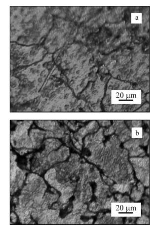
Fig. 10. Light microscope photographs of (a) aluminium and (b) iron compact.
