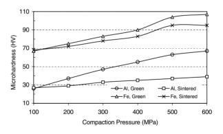
Fig. 11. Change of microhardness of powders before and after sintering under pressures.
