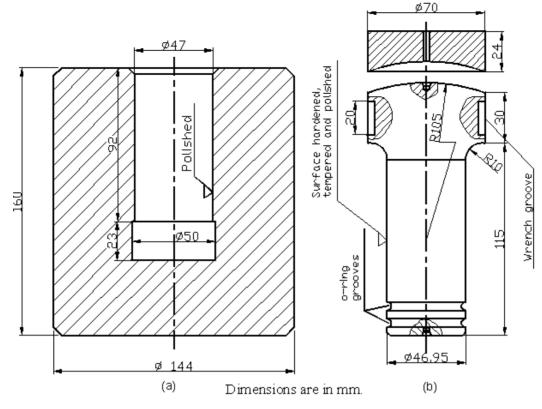
Fig. 2. Wet Bag CIP unit used: (a) pressure body, (b) compression piston.
