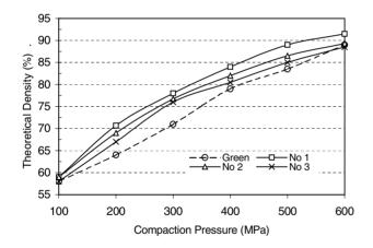
Fig. 6. Comparison of % densities of green and sintered Fe compacts.
