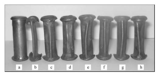
Fig. 4. The deformation of the flexible container under applied pressures: (a) before pressing, (b) empty pressing (20 MPa), (c) 100 MPa, (d) 200 MPa, (e) 300 MPa, (f) 400 MPa, (g) 500 MPa, (h) 600 MPa.
