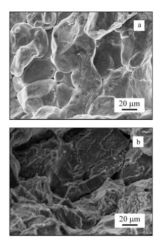
Fig. 8. SEM micrographs of the Al specimens: (a) before sintering, (b) after sintering.
