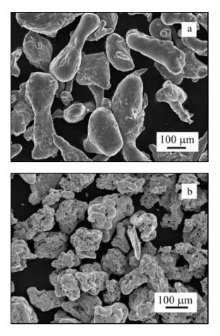
Fig. 7. The photographs of SEM before compaction: (a) Fe, (b) Al.
