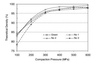
Fig. 5. Comparison of % densities of green and sintered Al compacts.
