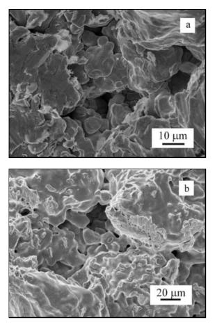
Fig. 9. SEM micrographs of the Fe specimens: (a) before sintering, (b) after sintering.
