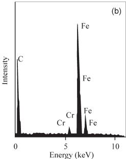
Fig. 5. SEM microfractograph of low-alloyed CrMoNb steel weld metal after Charpy impact testing (a) and EDX spectrum of carbide particle (b).
