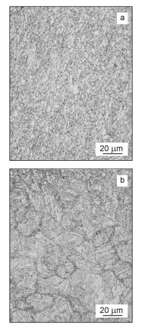
Fig. 1. Micrograph of the low-alloyed CrMoNb steel, LM, a) base metal, b) heat-affected zone/base metal interface.
