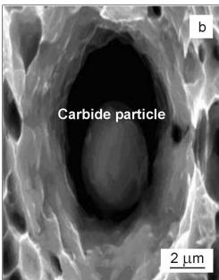
Fig. 6. SEM microfractographs of low-alloyed CrMoNb steel weld metal after tensile testing. Specimens annealed at  $475\,^{\circ}\text{C}$ , a) basic view, b) detail.
