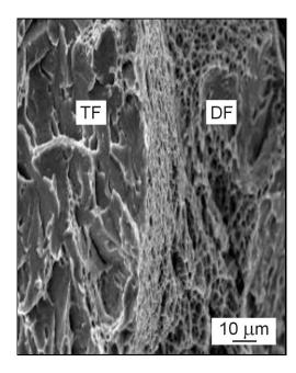
Fig. 4. SEM microfractograph of low-alloyed CrMoNb steel weld metal after Charpy impact testing. TF – transgranular cleavage, DF – areas of dimple morphology.
