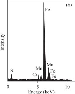
Fig. 7. SEM microfractograph of low-alloyed CrMoNb steel weld metal after tensile testing. a) Specimens annealed at 700  $^{\circ}$ C and b) EDX spectrum of non-metallic inclusion.
