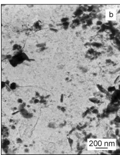
Fig. 3. Micrographs of low-alloyed CrMoNb steel weld metal, bright field images, TEM, a) I position, b) II position.
