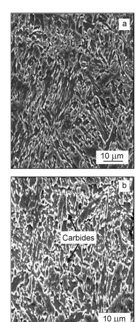
Fig. 2. SEM micrographs of low-alloyed CrMoNb steel weld metal, a) before PWHT, b) after PWHT.
