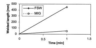
Fig. 8. Comparison of FSW and MIG welding processes for welding speed.
