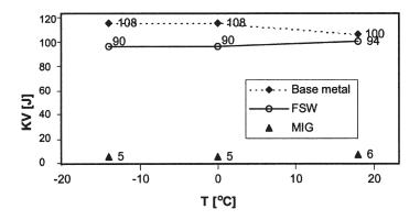
Fig. 5. Impact strength of FSW, MIG and base metal (FSW: friction stir weld, MIG: metal inert gas arc welding, base metal: EN AW-2014 (AlCu<sub>4</sub>SiMg) aluminium alloy).
