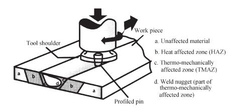
Fig. 1. Friction stir welding principle and microstructure [1].
