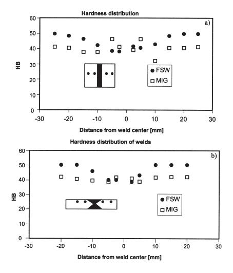
Fig. 6. Hardness distribution of FSW and MIG welded specimens (a - on the surface of weld, b - on the cross section of weld).
