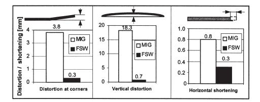
Fig. 7. The amount of distortion/shortening in FSW and MIG welding.
