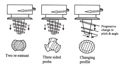
Fig. 2. Basic variants of FSW tools for welding thick work-pieces [3].
