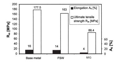
Fig. 4. Comparison of mechanical properties of FSW, MIG and base metal (FSW: friction stir weld, MIG: metal inert gas arc welding, base metal: EN AW-2014 (AlCu<sub>4</sub>SiMg) aluminium alloy).
