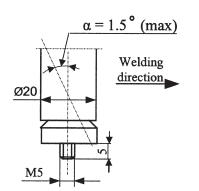
Fig. 3. Rotating tool details used in experiments (dimensions in mm, tool material: stainless steel).
