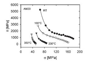
Fig. 2. Stress dependence of the work hardening rate; experimental data (points) fitted by the predicted equation (solid lines).
