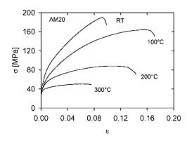
Fig. 1. True stress-true strain curves of AM20 polycrystals deformed at  $6.2 \times 10^{-5}$  s<sup>-1</sup> at various temperatures.
