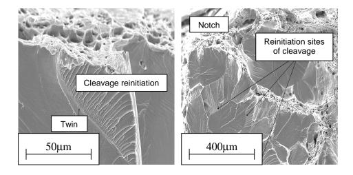
Fig. 15. Initiation of cleavage ahead of the ductile crack growth region.
