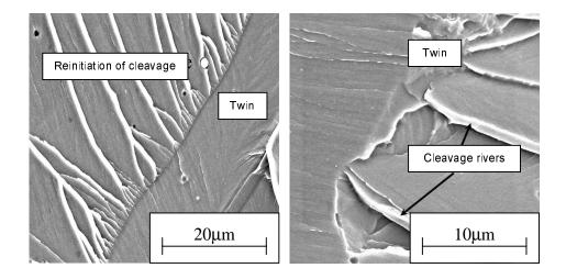
Fig. 5. Cleavage rivers terminated by the twin boundary.
