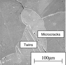
Fig. 7. Strong tendency to deformation twinning in the area of PCMCs.
