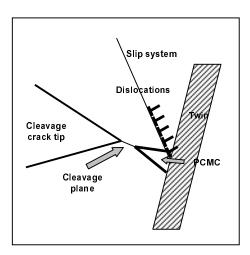
Fig. 17. Schematic representation of cleavage fracture.
