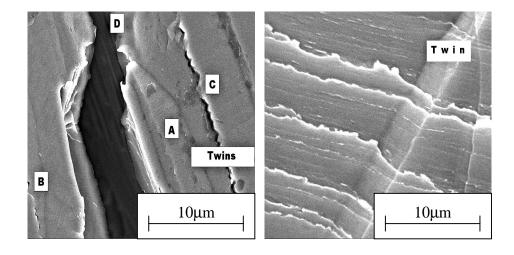
Fig. 3. Different stages of crack nucleation on the twin boundary.
