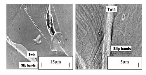
Fig. 1. Twin boundary acting as an obstacle for slip dislocations.
