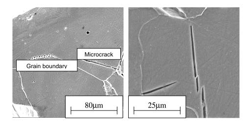
Fig. 11. Complex nature of the failure in the vicinity of the main crack.
