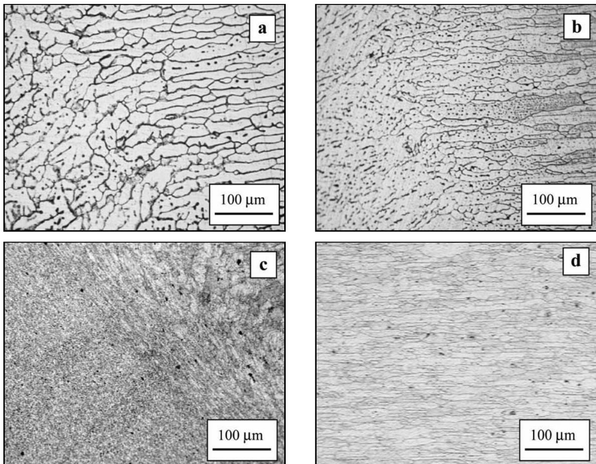
Fig. 3. Base metal to weld metal transition region: (a) TIG, (b) MIG, (c) FS welded specimen, (d) microstructure of base metal AA 7075.
