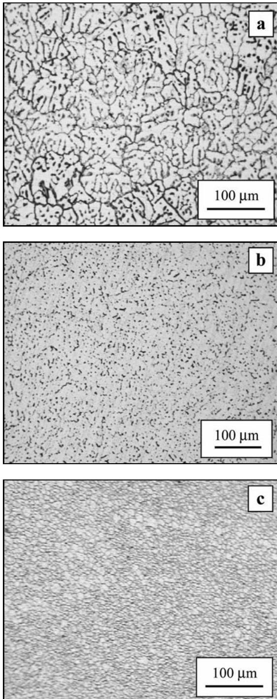
Fig. 4. Microstructure of weld centre: (a) TIG, (b) MIG, (c) FS welded specimen.
