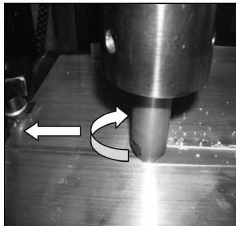
Fig. 1. Schematic view of FSW process.
