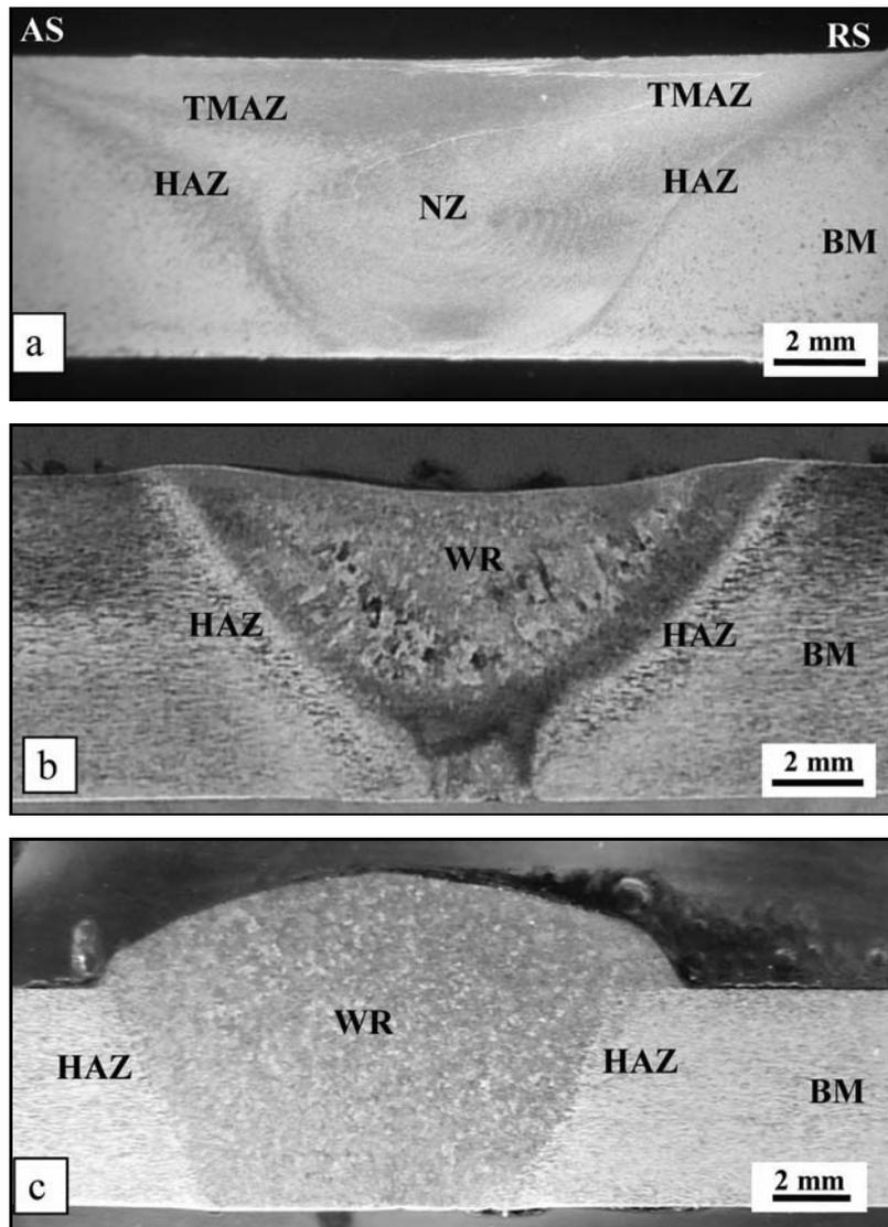
Fig. 2. Cross section of joints depicting the various zones formed as a result of (a) FSW, (b) TIG welding, (c) MIG welding.
