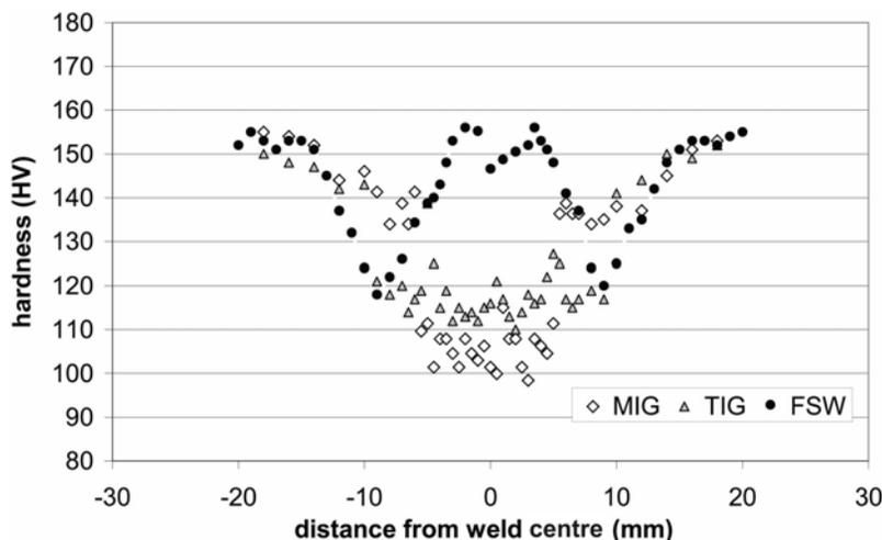
Fig. 5. Hardness profiles of weld cross section of TIG, MIG and FS welded AA 7075.
