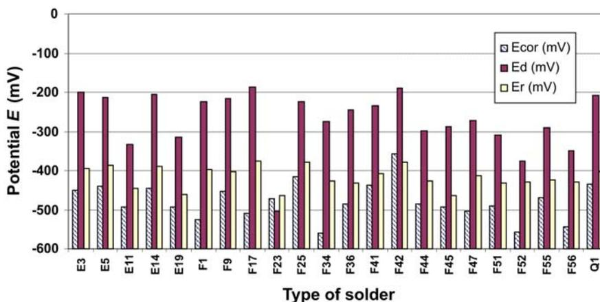
Fig. 5. Comparison of potentials of pitting corrosion for the studied solder types in 0.1 M NaCl solution.  $E_{cor}$  is corrosion (free) potential,  $E_d$  is potential of depassivation,  $E_r$  is potential of repassivation.
