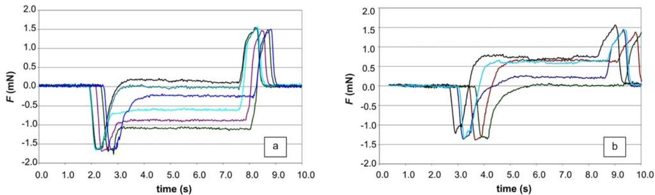
Fig. 2. Examples of the curves of wettability measurements (Cu wire diameter 1.0 mm, flux Epsilon 5),  $F$  is wetting power. a) copper/Sn95.5Ag3.8Cu0.7, b) copper/Sn63Pb37.
