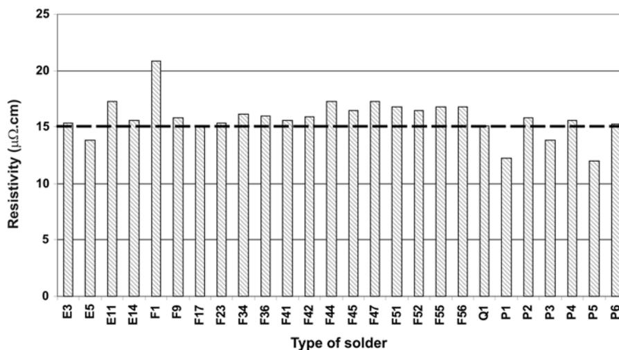
Fig. 4. Comparison of resistivity of the solders.
