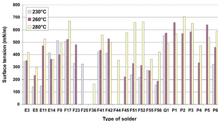
Fig. 3. Comparison of surface tensions of individual solders at the temperatures 230°C, 260°C and 280°C.
