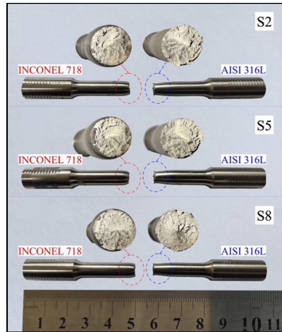
Fig. 6. S2, S5, and S8 tensile specimens and rupture surfaces.
