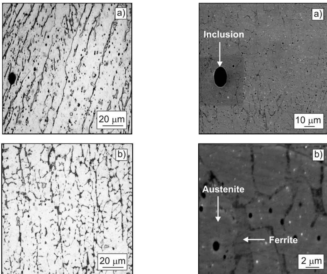
Fig. 5. Optical micrograph of AISI 316L stainless steel weld metal before PWHT (a) and after PWHT at 800°C (b).
