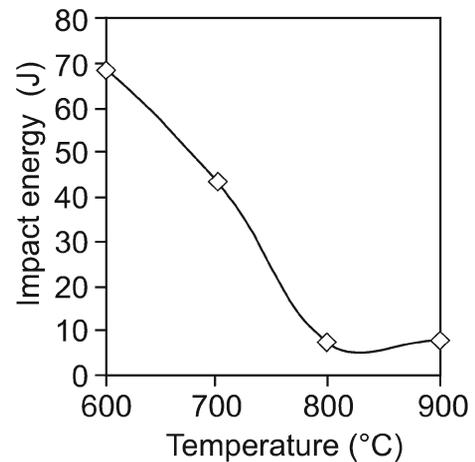
Fig. 1. Effect of annealing temperature on tensile strength (a), area reduction (b) and impact energy (c) of the weld metal.
