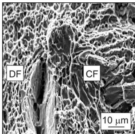
Fig. 8. SEM microfractograph of AISI 316L austenitic stainless steel weld metal after Charpy impact testing. DF – ductile fracture, CF – cleavage fracture.
