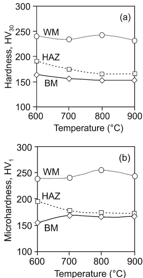
Fig. 3. Effect of annealing temperature on hardness (a) and microhardness (b) of the base metal (BM), the heat-affected zone (HAZ) and the weld metal (WM).
