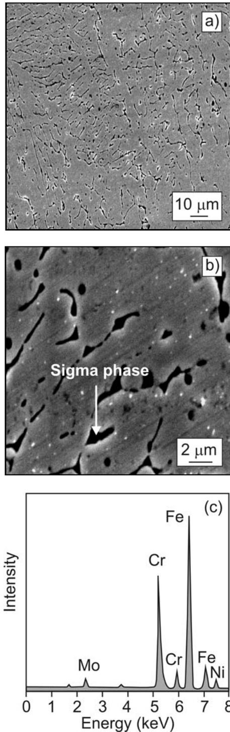
Fig. 7. SEM micrograph of AISI 316L stainless steel weld metal after PWHT at 800°C: a) basic view, b) detail, c) EDX spectrum of the sigma phase.
