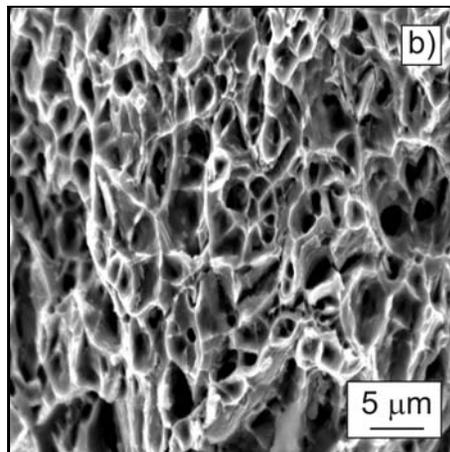
Fig. 9. SEM microfractograph of AISI 316L austenitic stainless steel weld metal after tensile testing: a) basic view, b) detail. Specimens annealed at 600°C.
