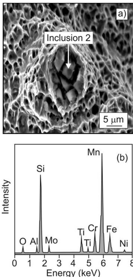
Fig. 11. SEM microfractograph of AISI 316L austenitic stainless steel weld metal after Charpy impact testing (a) and EDX spectrum of complex Mn-Cr-Si-Ti inclusion (b). Specimens annealed at 800°C.
