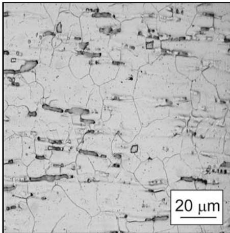
Fig. 4. Optical micrograph of AISI 316L stainless steel base metal.
