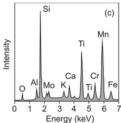
Fig. 6. SEM micrograph of AISI 316L stainless steel weld metal before PWHT: a) basic view, b) detail, c) EDX spectrum of the microslag inclusion.
