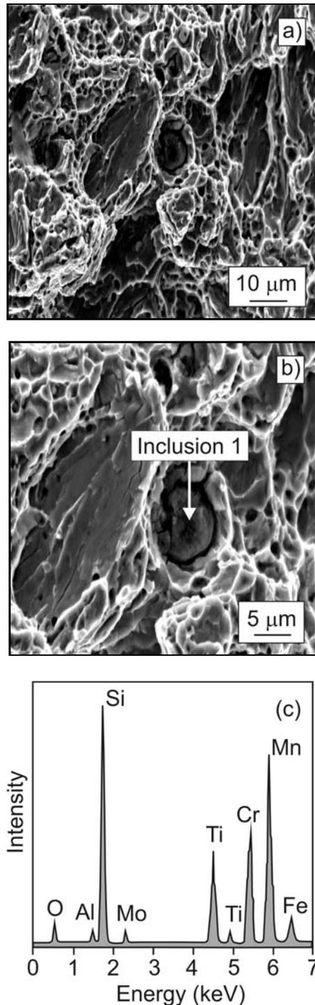
Fig. 10. SEM microfractograph of AISI 316L austenitic stainless steel weld metal after tensile testing: a) basic view, b) detail, c) EDX spectrum of complex Mn-Cr-Si-Ti inclusion. Specimens annealed at 800 °C.
