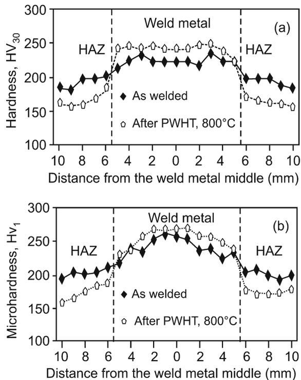
Fig. 2. Distribution of Vickers hardness  $HV_{30}$  (a) and microhardness  $HV_1$  (b) of welded parts after welding and after PWHT.
