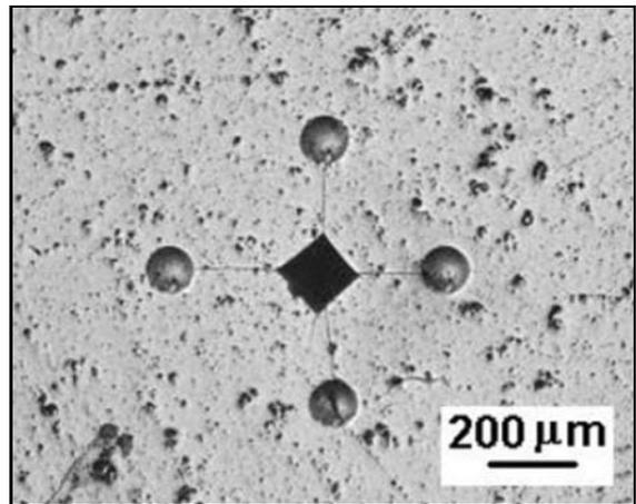
Fig. 1. Specimen with the primary Vickers indent and indentation cracks and secondary impressions by Rockwell ball causing very localized deformation at the original crack tips.
