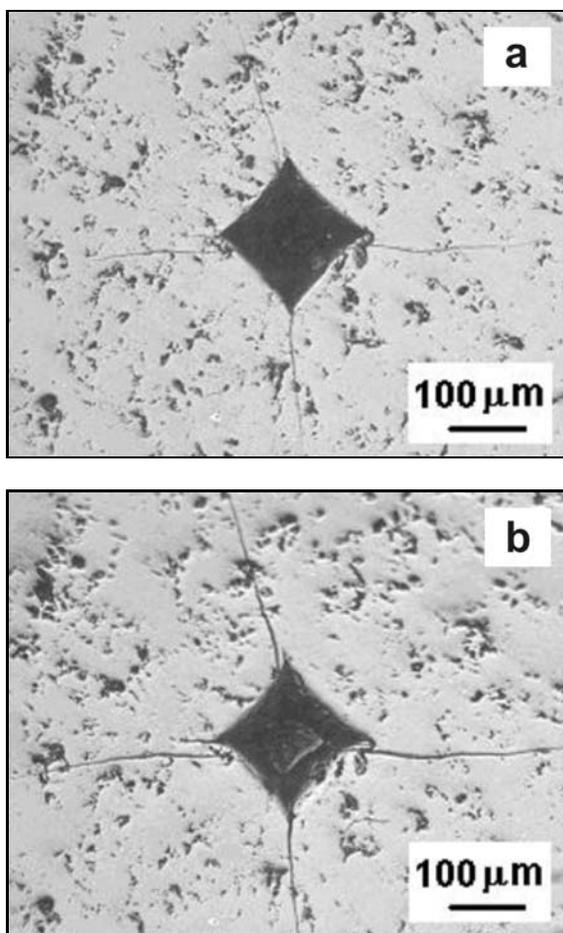
Fig. 8. Primary cracks growth by the specimen No. 19, couple No. 10: (a) initial state, (b) after 8 cycles.
