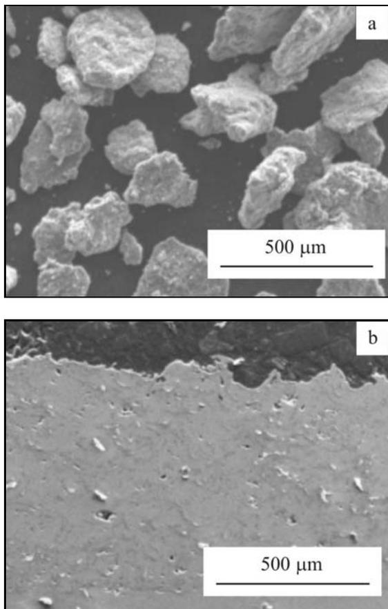
Fig. 1. (a) powder morphology after mechanical alloying, (b) typical microstructure of the coating.
