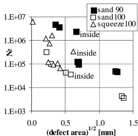
Fig. 14. Dependence of lifetime  $N_f$  on the initiation defect area square rooted.
