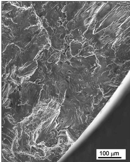
Fig. 7. Region labelled A with relatively flat fracture surface.
