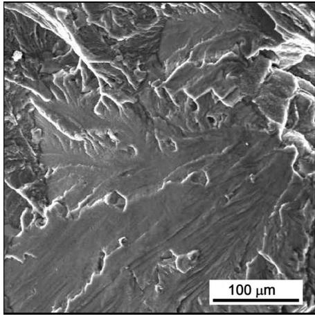
Fig. 10. Fatigue fracture facet with river pattern (region B).
