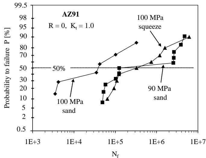
Fig. 3. Fatigue life distribution curves for sand cast and squeeze cast AZ91 alloy.
