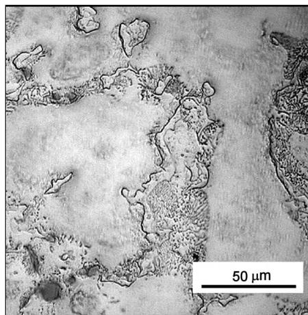
Fig. 2. Structure of squeeze-cast AZ91 alloy.
