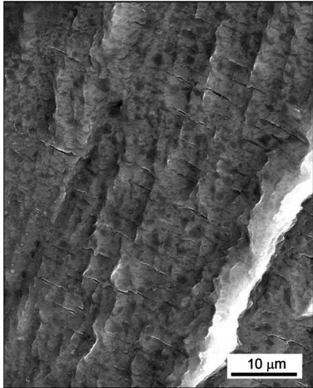
Fig. 12. Detail view on region C. Fracture facets with network of parallel microcrack.
