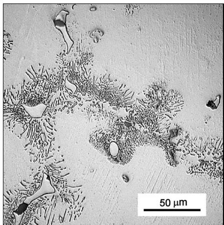
Fig. 1. Structure of sand-cast AZ91 alloy.
