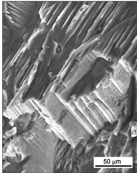
Fig. 9. Fatigue fracture facet with serrations and steps morphology (region B).
