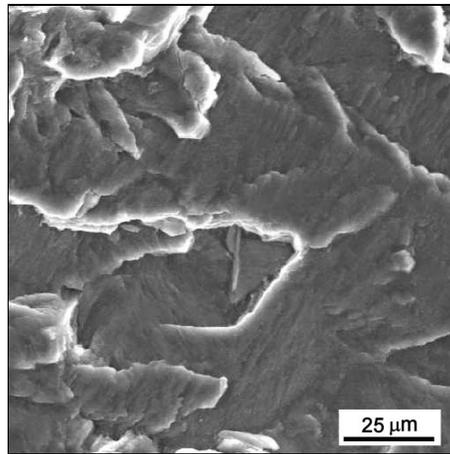
Fig. 13. Tiny, not very marked, fatigue striations on fracture surface in region C.
