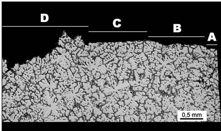
Fig. 6. Perpendicular section through fracture oriented in direction of fatigue crack propagation. Different regions are labelled. In bottom part of figure, latent crack is also shown.
