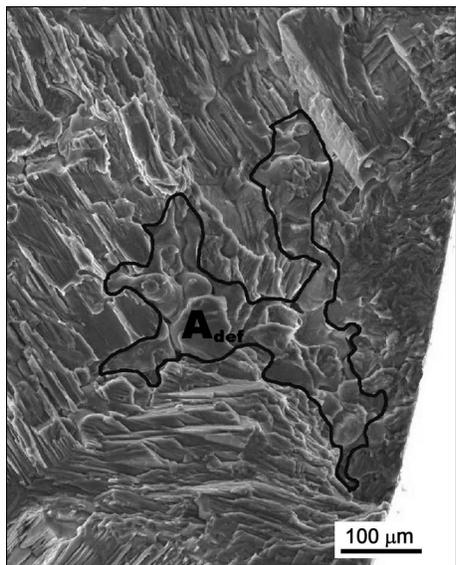
Fig. 4. Example of pore that acted as fatigue crack initiation site. Initiation defect area is labelled  $A_{def}$ .
