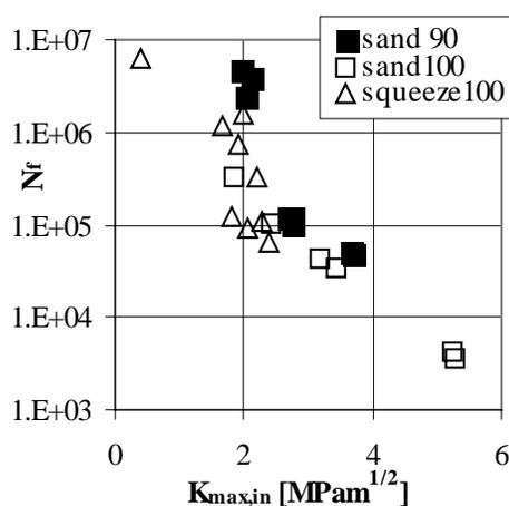
Fig. 15. Dependence of lifetime  $N_f$  on the maximum stress intensity factor  $K_{\max,\text{in}}$  in the tip of the initiation defect.
