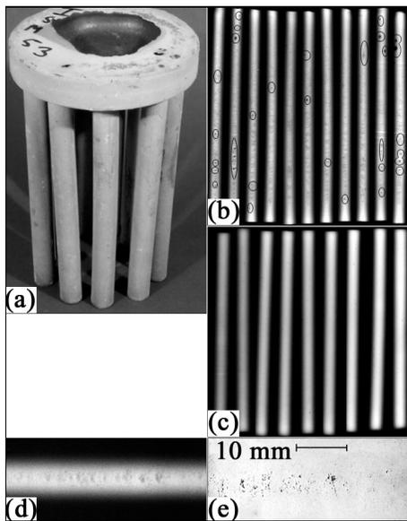
Fig. 7. (a) Typical top-gated mould used to cast 20 mm diameter bars (the pouring bush is missing); (b) isolated bubbles in bars cast in mould at 500 °C; (c) absence of major defects in bars cast in mould at 1000 °C; (d) radiograph and (e) macrosection showing layer porosity.
