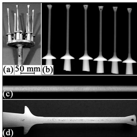
Fig. 13. (a) Mould of TiAl valves produced by counter-gravity casting; (b) radiograph showing absence of major defects in valve heads and stems; (c) digitally-enhanced radiograph of stem of valve #3 showing mottling; (d) macro-section through valve showing centreline interdendritic porosity. (NB the holes in the ends of the stems are in a 'flow-off' and not part of the final valve.)
