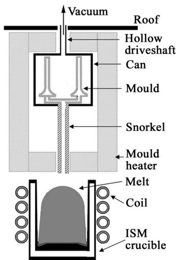
Fig. 10. Schematic view of the equipment used for counter-gravity casting TiAl components.
