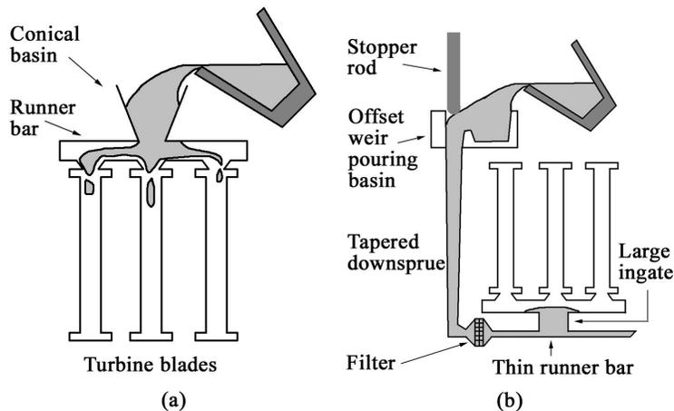
Fig. 6. Schematic mould designs for casting turbine blades using (a) top-gating and (b) bottom-gating.
