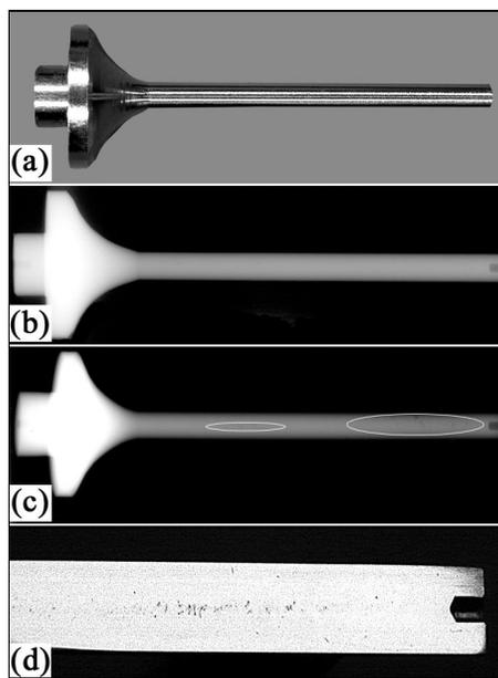
Fig. 15. Centrifugally-cast TiAl exhaust valves: (a) in machined condition; (b) radiograph showing absence of defects; (c) and (d) radiograph and macro-section showing fine centreline porosity.
