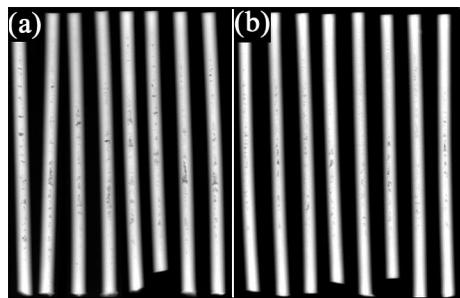
Fig. 14. 10 mm diameter TiAl bars centrifugally-cast in a multi-layer mould showing defects in (a) top layer; (b) bottom layer.
