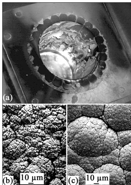
Fig. 3. (a) Deposits on ISM crucible after melting TiAl under vacuum; (b) SEM image of one area: 49 % Al, 42 % O, 8 % Mn (wt.%); (c) SEM image of another area: 85 % Al, 12 % Mn (wt.%).
