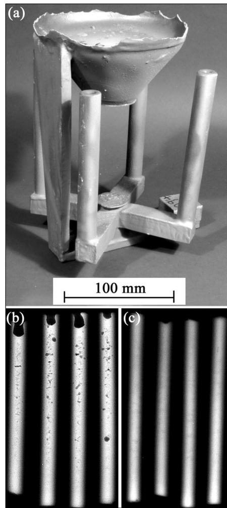
Fig. 8. (a) Bottom-gated mould used to cast 20 mm diameter bars; (b) extensive defects – mould temperature 500 °C; (c) defect-free bars – mould temperature 1300 °C.
