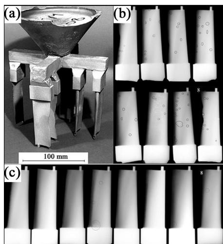
Fig. 9. (a) Top-gated mould of TiAl turbine blades; (b) many small bubbles formed with a mould temperature of 1000°C; (c) much improved quality with a mould temperature of 1300°C.
