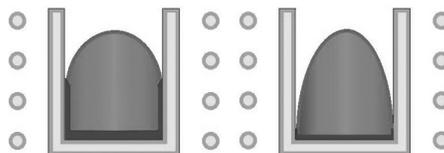
Fig. 2. Schematic views of (a) low power; (b) high power ISM furnaces.
