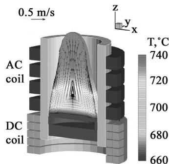
Fig. 5. Effect of superimposing a DC field (10 kA) on the flow and temperature in a 2.8 kg charge of Al alloy.
