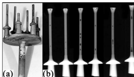
Fig. 12. Counter-gravity cast TiAl valves: (a) incompletely-filled mould due to too low a differential pressure; (b) radiograph showing turbulence-induced bubbles due to too high a differential pressure.
