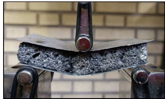
Fig. 4. Foam core sandwich beam under three-point bending test.
