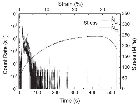
Fig. 3. Stress-strain and AE count rate-time curves of 5754 alloy, position 1.
