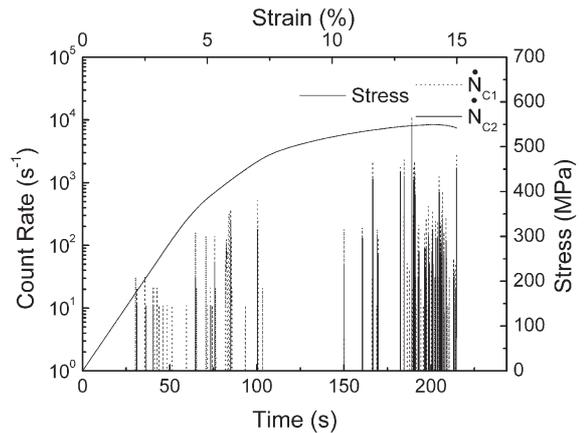
Fig. 7. Stress-strain and AE count rate-time curves of 1441 alloy, position 4.
