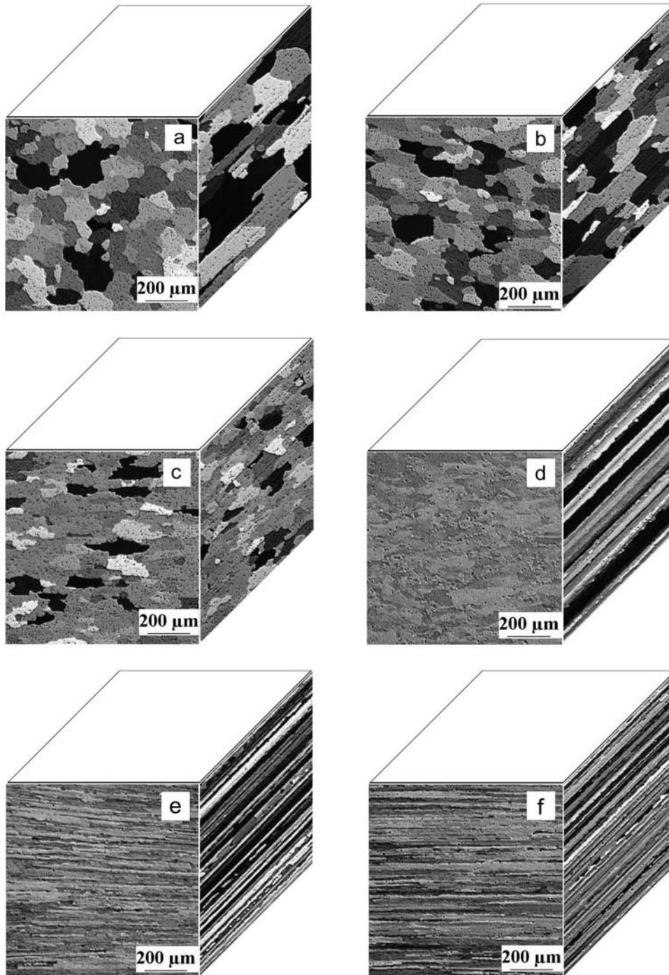
Fig. 2. Micrographs of aluminium alloys: AlMg3 from a) position 1, b) position 2, c) position 3 and AlCuMgLi from d) position 1, e) position 2, f) position 3.
