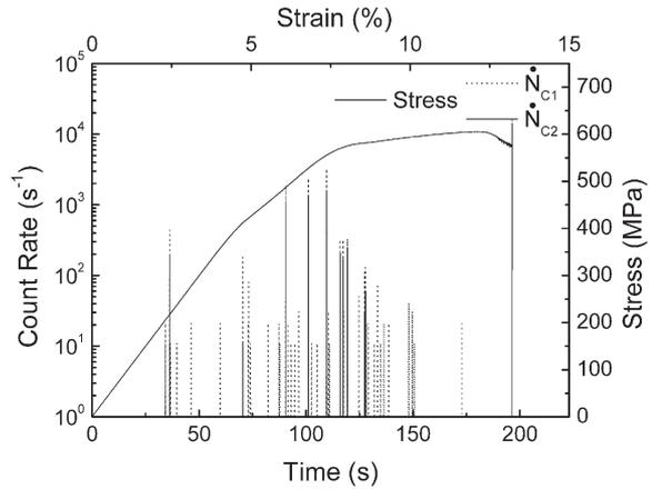
Fig. 5. Stress-strain and AE count rate-time curves of 1441 alloy, position 1.
