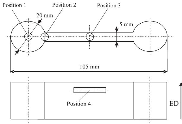
Fig. 1. Schematical drawing of extruded profile with setting out of sample positions.
