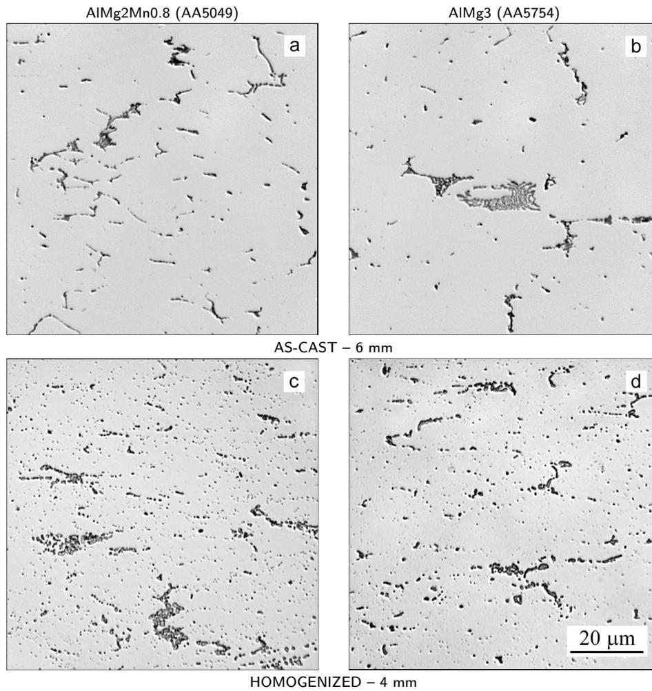
Fig. 1. Second-phase particles in studied Al-Mg sheets in the as-cast (a) (b) and homogenized condition (c) (d).
