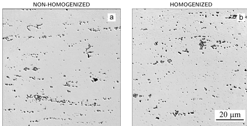
Fig. 3. Second-phase particles in non-homogenized (a) and homogenized (b) sheet of the AlMg3 (AA5754) alloy at the final gauge 1.0 mm.
