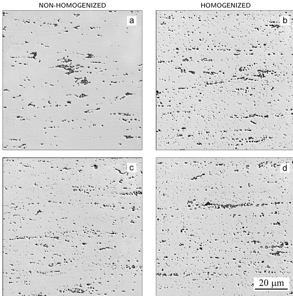
Fig. 2. Second-phase particles in non-homogenized (a) (c) and homogenized (b) (d) sheets of the AlMg2Mn0.8 (AA5049) alloy at the final gauge 1.0 mm.
