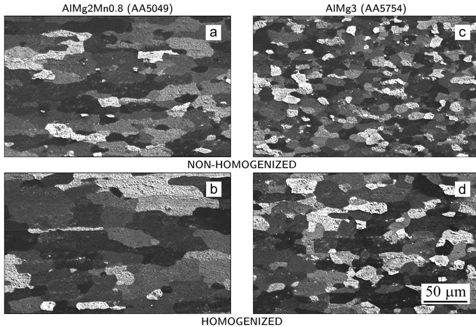
Fig. 4. Grain structure of non-homogenized (a) (c) and homogenized (b) (d) Al-Mg sheets at the final gauge 1.0 mm.
