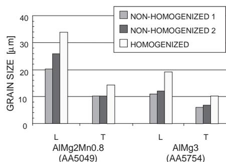
Fig. 5. Grain size of the 1.0 mm gauge sheets in the long transverse plane (L – rolling direction, T – transverse direction).
