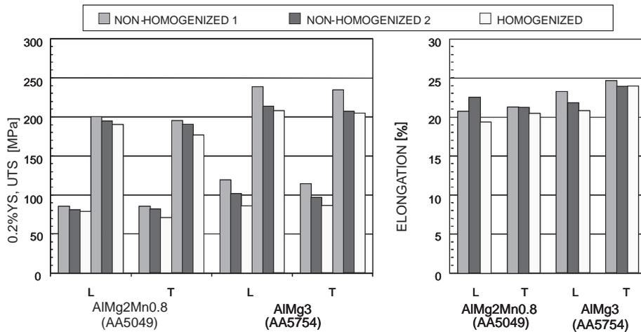
Fig. 6. Tensile mechanical properties of annealed 1.0 mm gauge sheets (O-temper).
