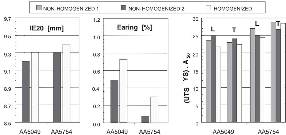
Fig. 7. Height of Erichsen dome (IE20), results of the cupping test (Earing) and formability parameter (UTS-YS).A<sub>50</sub> of annealed 1.0 mm gauge sheets (O-temper).
