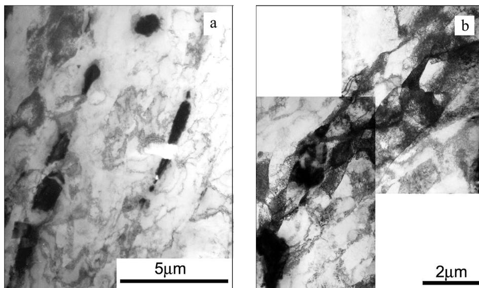
Fig. 5. TEM micrograph of cold rolled structure of the alloy-oval primary phases (a), subgrains (b).
