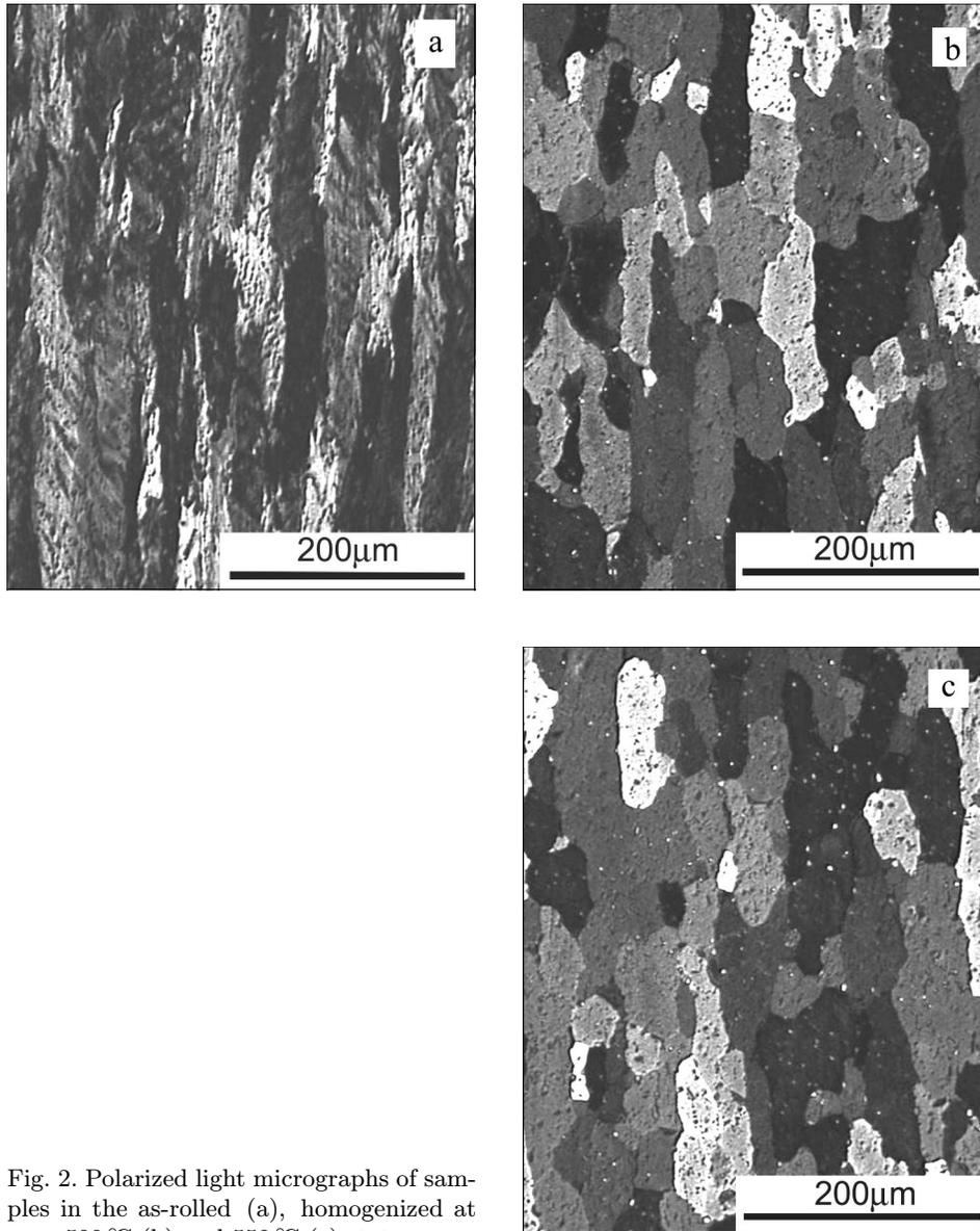
Fig. 2. Polarized light micrographs of samples in the as-rolled (a), homogenized at 500 °C (b) and 550 °C (c) states.
