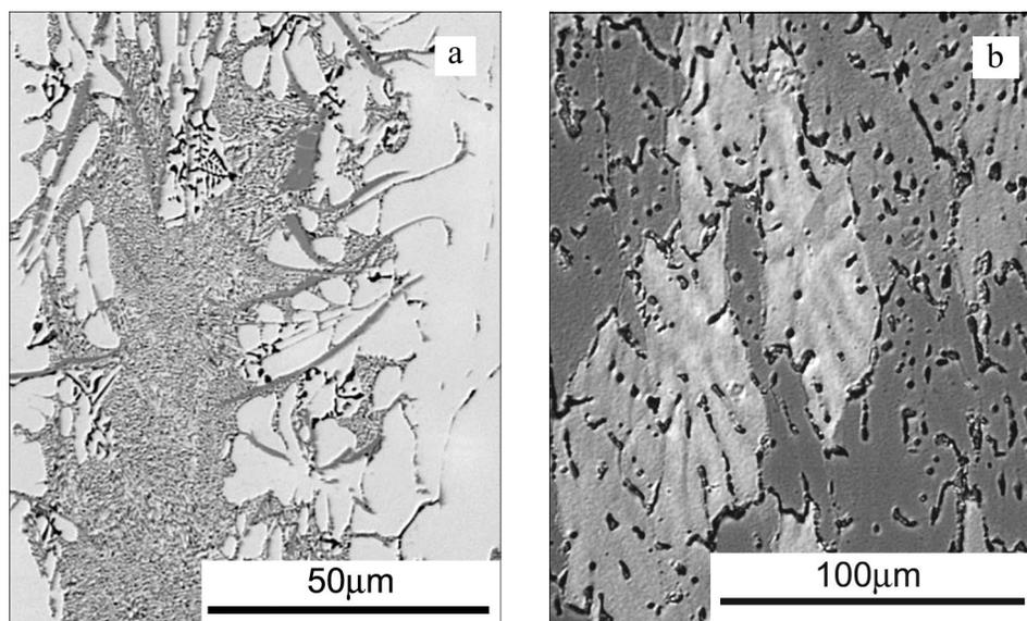
Fig. 1. Light microscopy micrograph of CLSC (a) and grain in the as-cast alloy (b).
