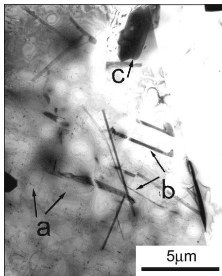
Fig. 6.  $Mg_2Si$  precipitates in sample homogenized to 500 °C: a) fine  $\beta''$  needles, b) coarser  $\beta'$  rods, c)  $Al_{12}(Mn,Fe)_3Si$  particle.
