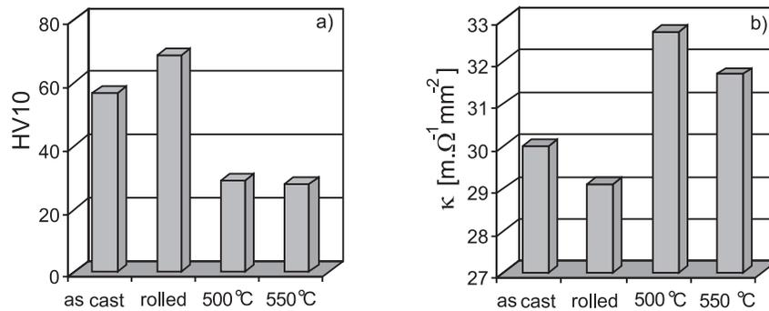
Fig. 3. Hardness (a) and conductivity (b) changes due to rolling (37% reduction), homogenization at 500 °C and 550 °C, respectively.
