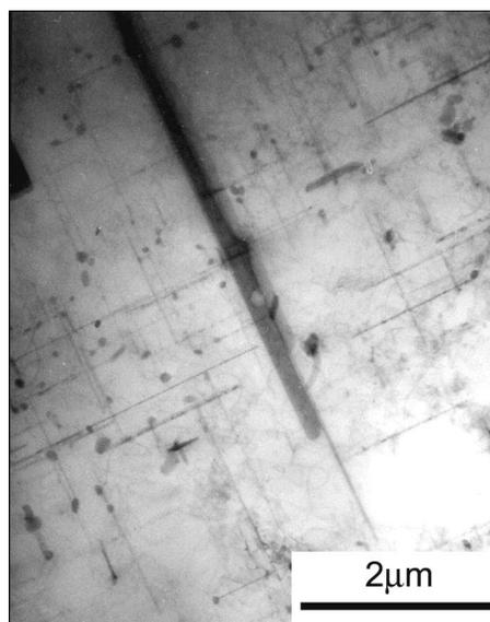
Fig. 7.  $\beta'$ - $Mg_2Si$  rods in sample homogenized to 550 °C.
