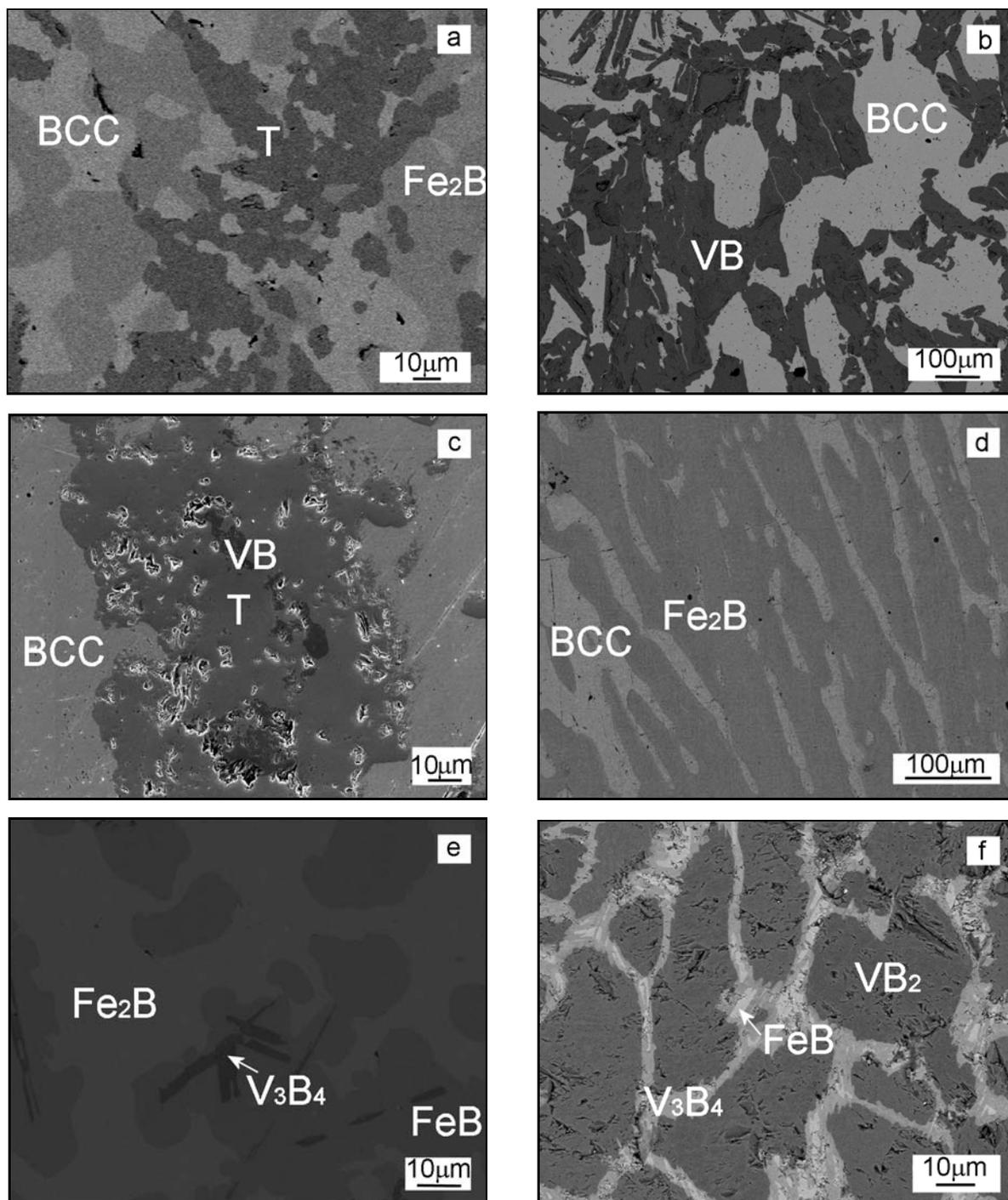
Fig. 1. Microstructure of Fe-B-V alloys (chemical composition of alloys is in at.%) after annealing at 1353 K for 60 days: a) 45Fe-34B-21V, b) 57Fe-20B-23V, c) 67Fe-18B-15V, and at 903 K for 190 days: d) 73Fe-25B-2V, e) 50Fe-45B-5V, f) 16Fe-60B-24V.
