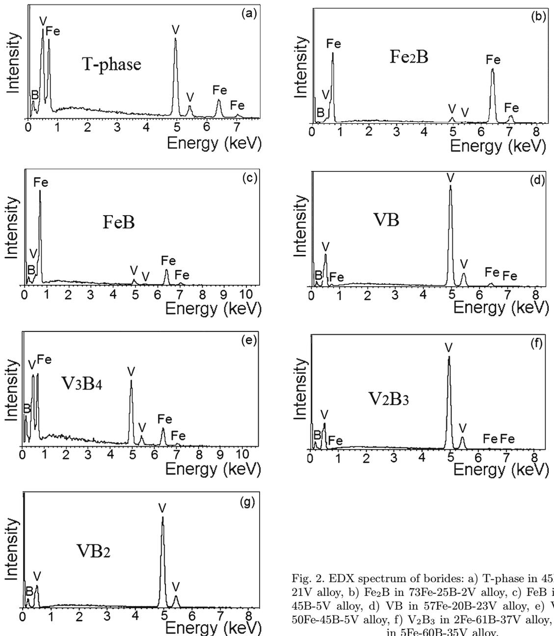
Fig. 2. EDX spectrum of borides: a) T-phase in 45Fe-34B-21V alloy, b) Fe<sub>2</sub>B in 73Fe-25B-2V alloy, c) FeB in 50Fe-45B-5V alloy, d) VB in 57Fe-20B-23V alloy, e) V<sub>3</sub>B<sub>4</sub> in 50Fe-45B-5V alloy, f) V<sub>2</sub>B<sub>3</sub> in 2Fe-61B-37V alloy, g) VB<sub>2</sub> in 5Fe-60B-35V alloy.
