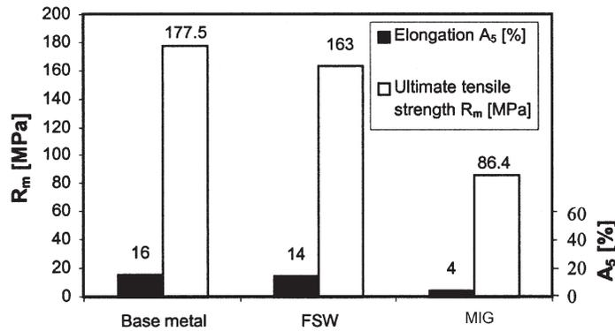
Fig. 4. Comparison of mechanical properties of FSW, MIG and base metal (FSW: friction stir weld, MIG: metal inert gas arc welding, base metal: EN AW-2014 (AlCu<sub>4</sub>SiMg) aluminium alloy).
