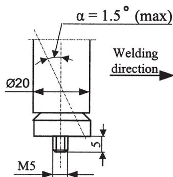
Fig. 3. Rotating tool details used in experiments (dimensions in mm, tool material: stainless steel).
