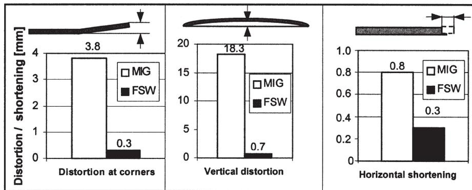
Fig. 7. The amount of distortion/shortening in FSW and MIG welding.
