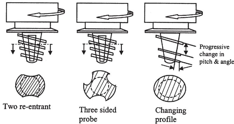
Fig. 2. Basic variants of FSW tools for welding thick work-pieces [3].
