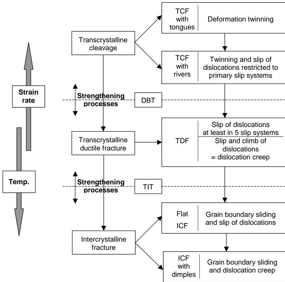
Fig. 1. Schematic representation of the relation between the deformation modes and fracture modes of ferritic steels.
